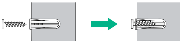
Figure 9 Driving a screw into a wall anchor
