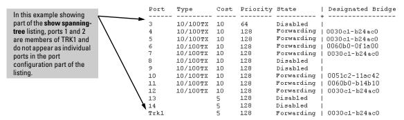
When Spanning Tree forwards on a trunk, all ports in the trunk will be forwarding. Conversely, when Spanning Tree blocks a trunk, all ports in the trunk are blocked.
