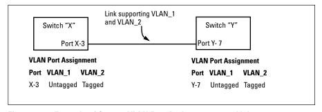
Figure 11-1. Example of Correct VLAN Port Assignments on a Link
