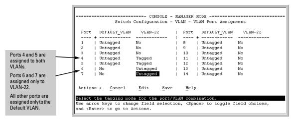
Figure 9-49. Example of VLAN Assignments for Specific Ports
