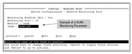
Figure 10-18.Example of Selecting a VLAN to Monitor
