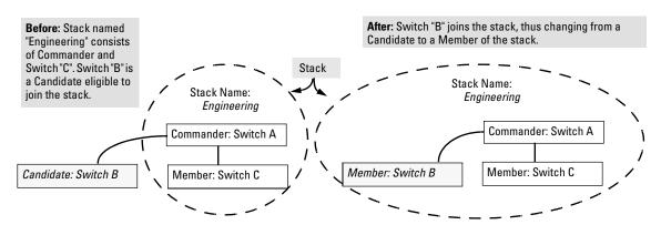
Figure 9-1. Illustration of a Switch Moving from Candidate to Member
