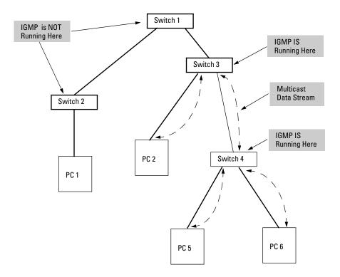
Figure 9-68. Isolating IP Multicast Traffic in a Network
