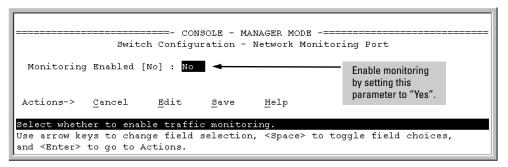
Figure 10-16. The Default Network Monitoring Configuration Screen
