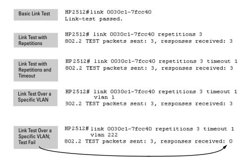
Figure 11-14.Example of Link Tests
