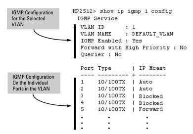
Figure 9-66. Example Listing of IGMP Configuration for A Specific VLAN
