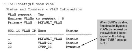
Figure 9-50. Example of "Show VLAN" Listing (GVRP Enabled)
