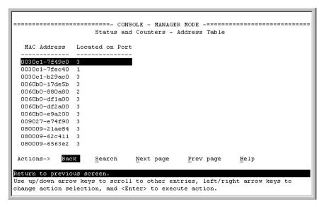
Figure 10-7. Example of the Address Table (Switch 4000M)
