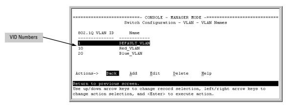
Figure 9-55. Example of VLAN ID Numbers Assigned in the VLAN Names Screen
