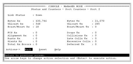
Figure 10-6. Example of the Display for Show details on a Selected Port
