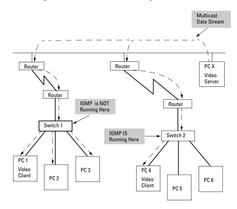
Figure 9-67. The Advantage of Using IGMP
