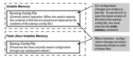
Figure C-10. Conceptual Illustration of Switch Memory Operation
