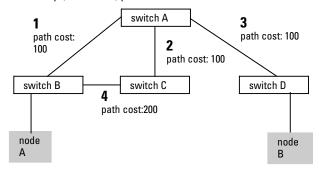
Figure 9-71. Example of Redundant Paths Between Two Nodes
