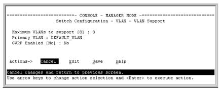
Figure 9-60. The VLAN Support Screen (Default Configuration)
