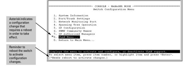
Figure 11-74.Indication of a Configuration Change Requiring a Reboot
