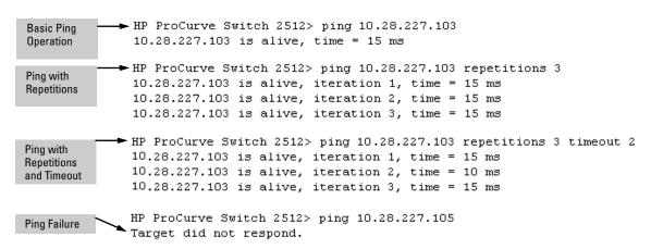
Figure 11-13.Examples of Ping Tests
