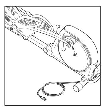
Next, remove the indicated M8 x 25mm Patch Screw (121), Large Axle Cover (113), M8 Washer (95), and Pedal Arm Sleeve (46). Using a flat screwdriver, carefully pry the left Disc (17) off the elliptical.
