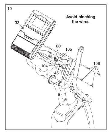
Attach the Front Upright Cover (24) to the Upright (5) with four M4 x 16mm Screws (106).
