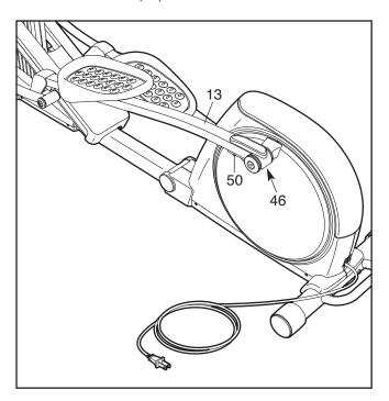
Next, remove the indicated M8 x 25mm Patch Screw (121), Large Axle Cover (113), M8 Washer (95), and Pedal Arm Sleeve (46). Using a flat screwdriver, carefully pry the left Disc (17) off the elliptical exerciser.
